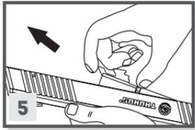
5. Remove the **barrel** from the **slide** by pulling to the front and up.
