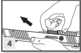
4. Release **slide spring assembly** from its position on the bottom of the **barrel**.
