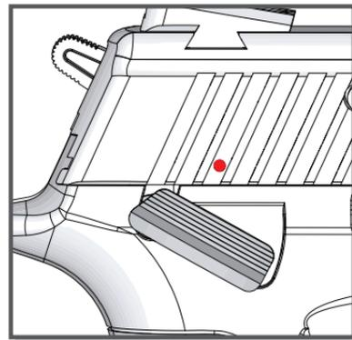
**4. Hammer Drop (Hammer Decocker).** This mechanism allows you to decock the hammer safely. The pistol remains ready to fire, in Double Action mode.
