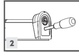
B) Slide the **magazine floor plate** toward the front of the magazine according to Position 1 and 2.
