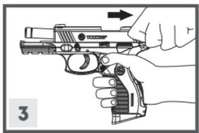
3. Hold the pistol with one hand keeping your finger away from the trigger and on the **memory pad**. With the other hand pull the **slide** backwards to its limit and release it. The slide will go forward under **recoil spring** pressure and will insert one cartridge in the chamber.
