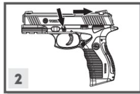
2. Hold the pistol according to figure 2A and with four fingers, keep the **slide** in its backward position approx. 1/8". Simultaneously, with the other hand's thumb and index finger, pull the
