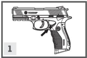
1. To remove the magazine, press the **magazine release button**, located near the **trigger guard**, with your thumb.
