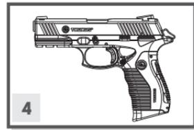
4. The pistol is now cocked and ready to fire by pulling the **trigger**. After firing, the **slide** will recoil from gas pressure and will eject the empty cartridge case and feed another cartridge into the chamber. The pistol will be ready to fire again. After the last round, the **slide** will remain in the open position held by the **slide catch**. In order to make it return to its rest position, press down on the **slide catch** just above the **left grip**.
