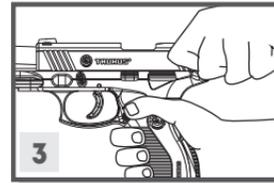
3. You should cycle the **slide** several times, with no magazine inserted and an empty chamber, to insure that the **barrel/slide/frame** relationship is correct.
