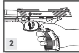
2. The **slide** should be mounted on the **frame** and pulled fully to the rear and the **slide catch** must be moved upward to hold the **slide** to the rear.
