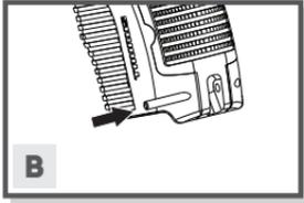
**B) REPLACEMENT:** to assemble the **backstrap**, adjust it to the **grip** and insert the **pin**. A tool can be used to make the assembling process easier.
