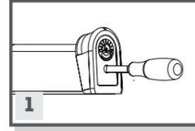
A) Use a **punch** to press in on **magazine spring seat/clip**.
