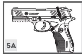
5. If you want to stop shooting before firing the last cartridge of a magazine, decock the firearm immediately by moving the **safety** downward (a) and push the safety lever in the up (on) position (b).
