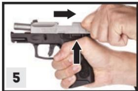
5. After the last round, the **slide** will remain in the open position held by the **slide catch**. In order to make it return to its rest position, press the **slide catch** downward just above the **left grip** or pull slide to the rear and let the slide go forward (you must remove the empty magazine first).
