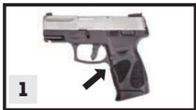
1. To remove the magazine press the **magazine release button**, located near the **trigger guard**, with your thumb.
