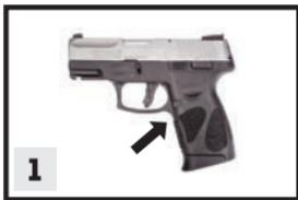
1. Before disassembly always (1) Keep your finger off or the **trigger** and on the **memory pad**, (2) point the **muzzle** in a safe direction (3) remove the **magazine** by pressing the **magazine release button** (4) pulling the **slide** to the rear and locking back and (5) looking and feeling the **magazine well** and **chamber** to confirm the pistol is empty. An empty firearm cannot fire.
