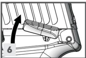
6. If you want to stop shooting before firing the last cartridge of a magazine, push the **safety lever** in the up (on) position or decock firing pin according to instructions on page 9.
