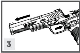
3. Pull and release **trigger**. Then remove the **slide** from the **grip**.
