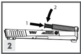
2. Insert the **spring/guide rod** sub-assembly into the **slide** over the barrel, compressing the **spring** slightly to get it into position.
