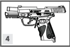
3 - 4. The **slide** should be mounted on the frame and pulled fully to the rear and the **slide catch** must be moved upward to hold the **slide** to the rear.
