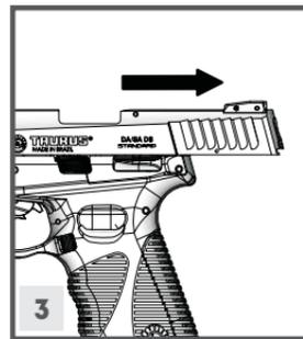
3. Hold the pistol with one hand keeping your finger away from the trigger. With the other hand pull the **slide** to its limit and release it, so **slide** will go forward under **recoil spring** pressure and will insert one cartridge in the chamber.
