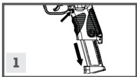
1. To remove the magazine press the **magazine release button**, located near the **trigger guard**, with your thumb.
