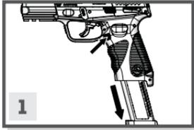
1. Remove the **magazine** by pressing the **magazine release button**.
