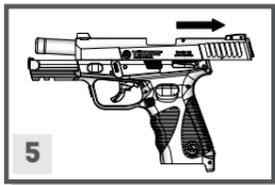
5. You should cycle the **slide** several times, with no **magazine** inserted and no rounds in the chamber, to insure that the barrel / slide / frame relationship is correct.
