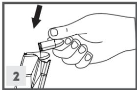
2. To load magazine hold the bottom of the **magazine** with one of your hands and with the other one insert the cartridges one at a time, pressing them down and to the rear. Insert the **magazine** into the pistol until it is held by the **magazine catch**. If the **magazine** is not correctly inserted into the pistol, it can be dropped when you intend to shoot.
