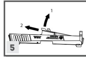
5. Remove the **barrel** from the **slide** by pulling it to the front and up.
