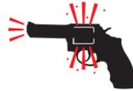
When firing any revolver be sure all persons are a safe distance to the rear of the shooter. When fired, all revolvers discharge hot gas and particles through the clearance gap between the cylinder and rear of the barrel during normal use.
