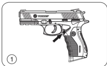
1. To remove the magazine press the **magazine release button**, located near the **trigger guard**, with your thumb.
