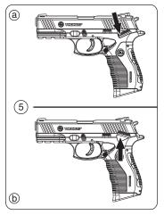
4. The pistol is now cocked and ready to fire by pulling the **trigger**. After firing, the **slide** will recoil from gas pressure and will eject the empty cartridge case and feed another cartridge into the chamber. The pistol will be ready to fire again. After the last round, the **slide** will remain in the open position held by the **slide catch**. In order to make it return to its rest position, press the **slide catch** just above the **left grip**.
