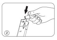
2. Hold the **magazine** with one of your hands and with the other one insert the cartridges one at a time, pressing them down and to the rear. Insert the **magazine** into the pistol until it is held by the **magazine catch**. If the **magazine** is not correctly inserted into the pistol, it can be dropped when you intend to shoot.
